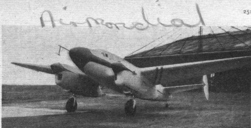
FRENCH EXPERIMENT: A recent photograph of the Rey 01 twin-engined light monoplane that reveals the extremely clean aerodynamic form of this French experimental aircraft. Two prototypes have been built, the first of which made its maiden flight on December 16th last.
