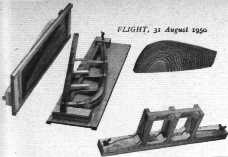
Router jigs, adjusting block and drill jig in Hydulignum, produced for the de Havilland Company by Hordern-Richmond, Ltd.
