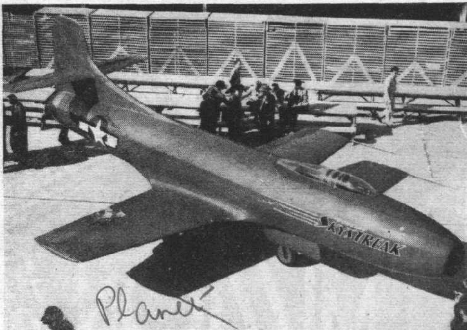
SKYSTREAK: One of the two new Douglas Skystreak transonic research machines. Built for the U.S. Navy the aircraft shown is alternatively designated D-558. A General Electric TG 180 axial-flow turbine jet is fed through a bifurcated duct from a nose intake. The wing area is 150 sq ft; wing loading 65 lb/sq ft (55 lb/sq ft at landing); span 25ft and length 35ft 1½in.
