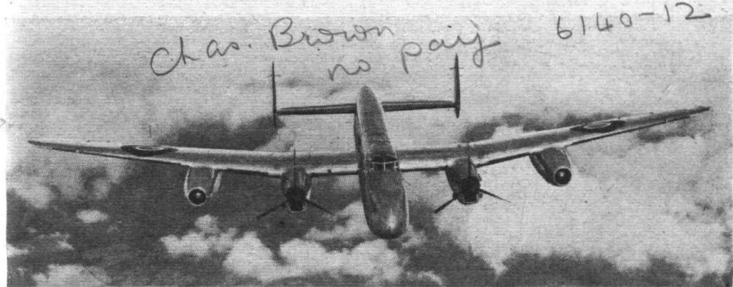
The Nene Lancasterian has a very good performance on the pure jet power of its two Nenes. Mr. R. T. Shepperd, Chief Test Pilot of the Rolls-Royce Flight Development and Testing Establishment at Hucknall, here demonstrates the Lancasterian with inboard Merlins feathered.
