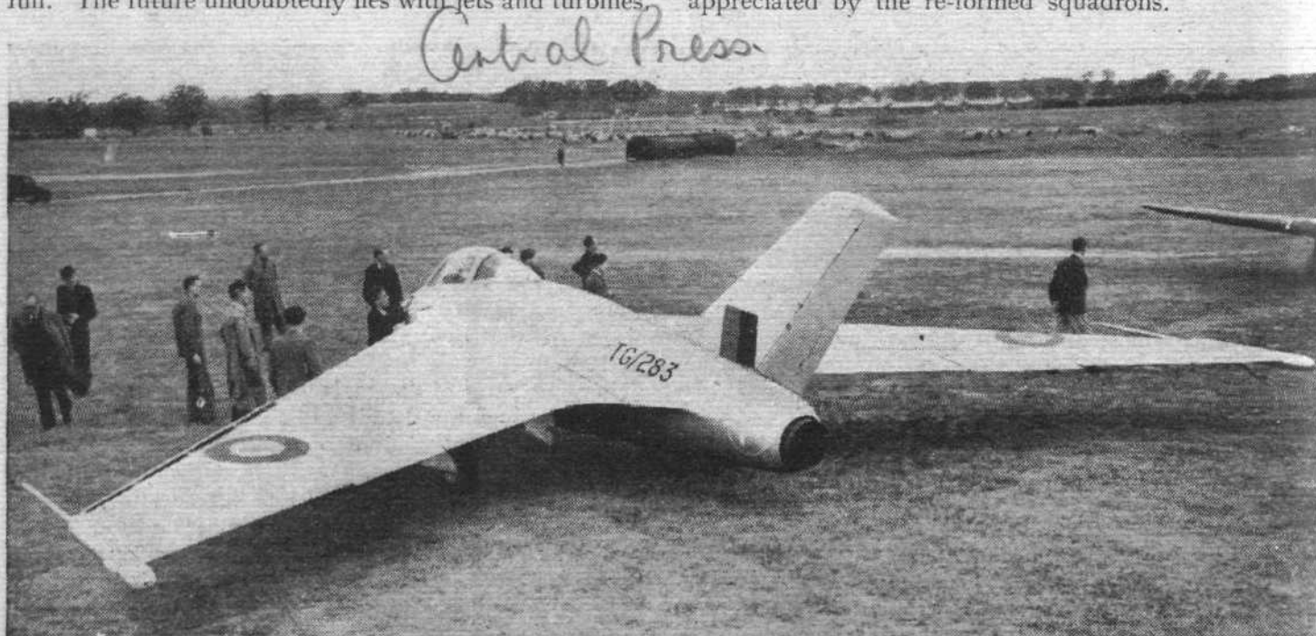
EXPLORATORY: The de Havilland 108 high-speed research aircraft, built solely for the investigation of control and stability problems associated with swept-back wings. The fuselage is that of a Vampire, but the wing, with its slots and "elevons," embodies design features which may eventually be reproduced in the D.H. 106, or Brabazon IV, transport. The D.H. 108 has been flying since May 15th at Woodbridge and Hatfield.
