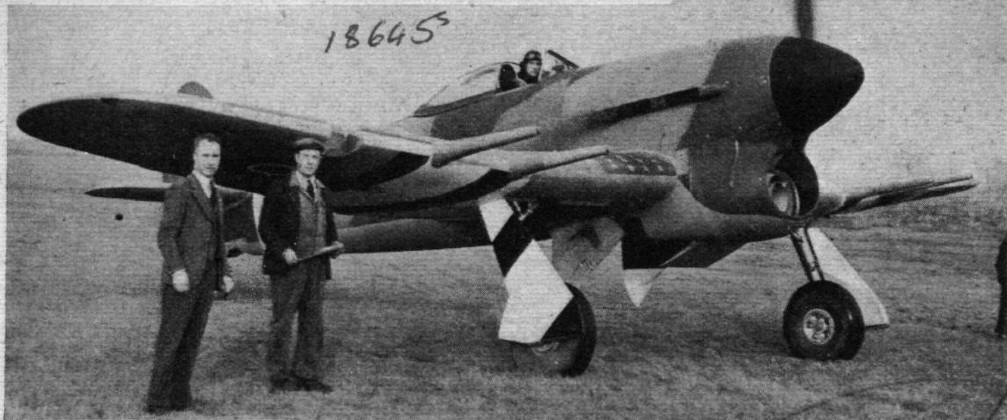
With the 2,200 h.p. Napier Sabre engine running, the "cleanness" of the nose become more apparent. The exhaust stubs each serve an upper and lower cylinder.
