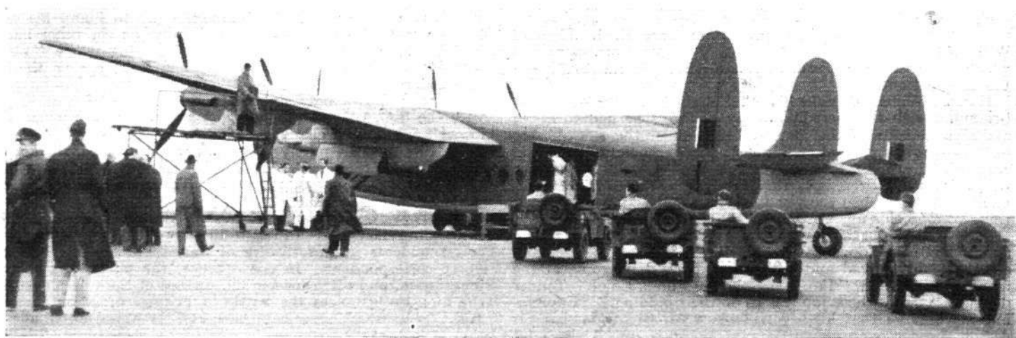
Four jeeps awaiting their turn for stowage. Each vehicle is driven up the ramp and into the fuselage where it is man-handled into position. The freight entrance is about 8ft. wide by 6ft. high.
