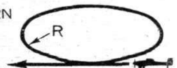
Fig. 23. Increase of control forces at high speeds in a turn.
