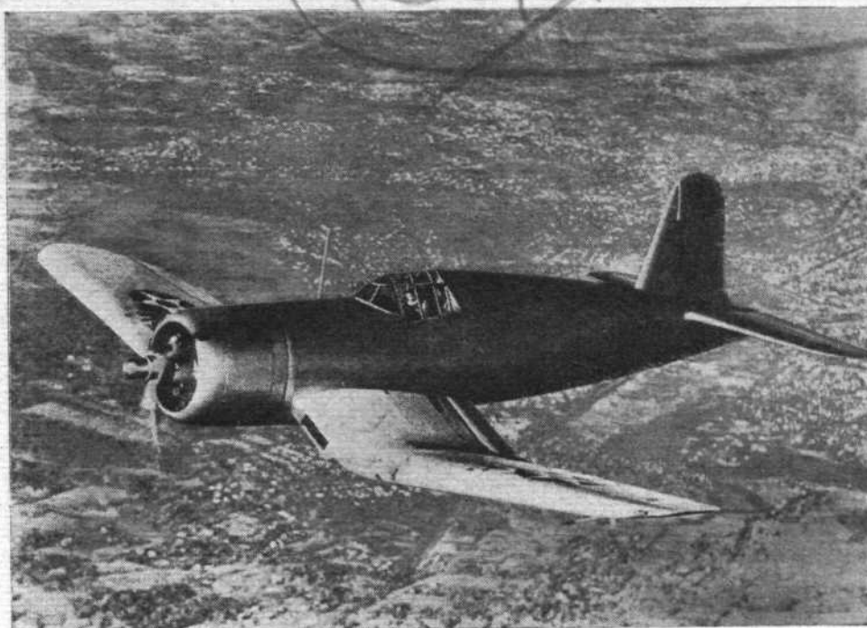
U.S. SHIPBOARD FIGHTER: The Vought-Sikorsky XF4U-1. A single-seater all-metal machine with an 18-cylinder Pratt & Whitney two-row radial of 1,850 h.p.
