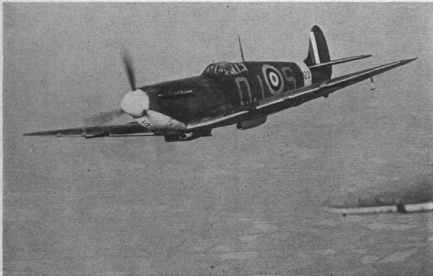
OFFENSIVE SWEEP'S BROOM: In the recent sweeps over Northern France the Mark V Spitfire has added to the laurels it already possessed as a metropolitan defender. This photograph, taken from a Blenheim, shows clearly the two 20 mm. shell-guns and four .303 machine guns. Of interest also is the D.H. constant-speed airscrew and the modified air intake and oil-cooler.
