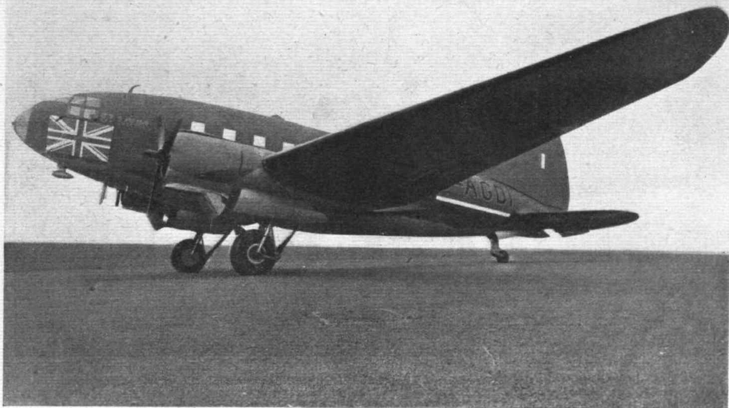
This three-quarter front view of the St. Louis gives a good idea of the large but beautifully streamlined fuselage and the long chord cowlings of the 18 cyl. double row Cyclone engines.
