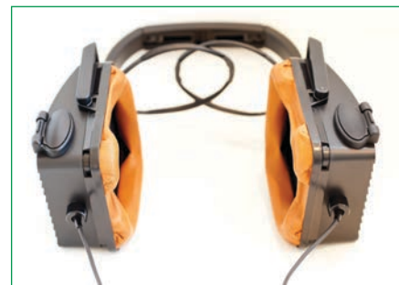
Photo 2: The TakeT H2 headphones’ design resolves the low-frequency problems of limited excursion by using a piezoelectric air motion transformer.
