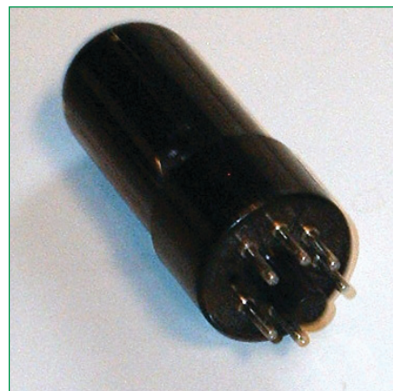
Photo 3: The 6V6 is basically a lower-power 6L6.
