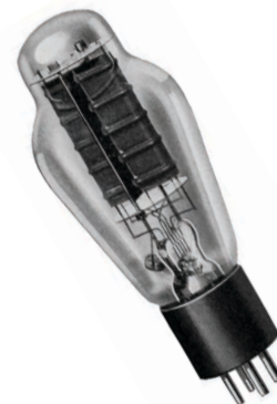
Photo 8: The Western Electric 300B is one of the most popular power triodes.
