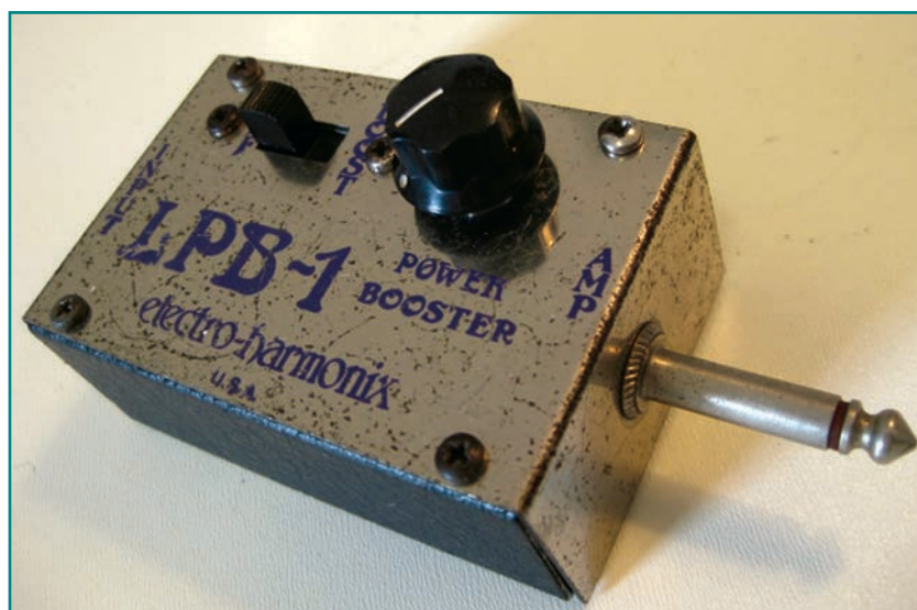
Photo 2: The Electro-Harmonix LPB-1, introduced in the late 1960s, boosted signal levels to overdrive amp input stages.
