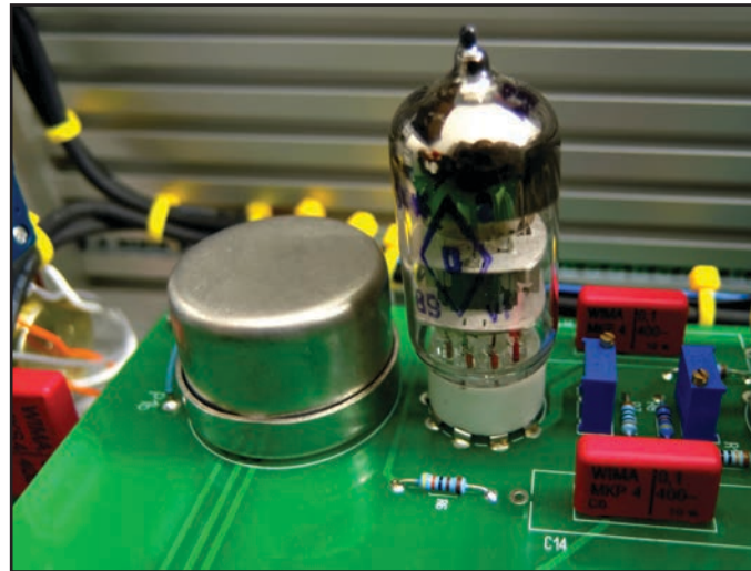
As an all-tube unit, the comp.two relies on one Electro-Harmonix 6CG7 vacuum tube and one new old stock (NOS) Russian-made 6N3P per channel.
