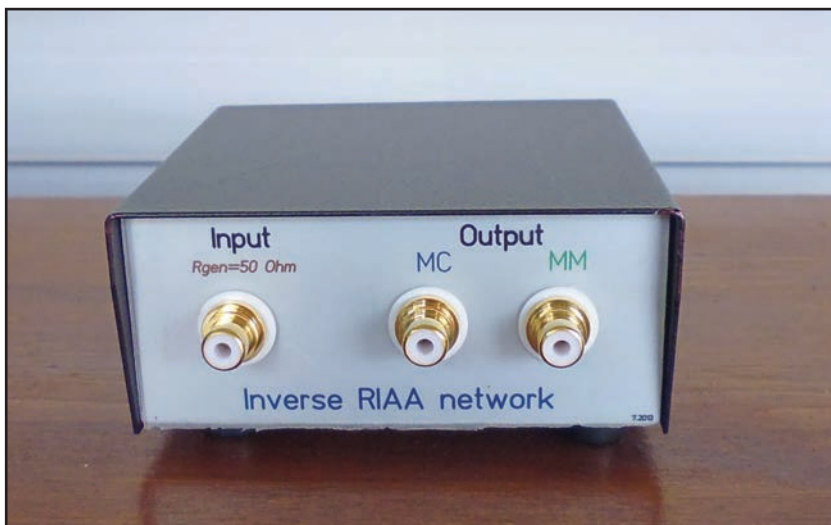
Photo 6: This enclosure contains the inverse RIAA network that I used for the measurements.
