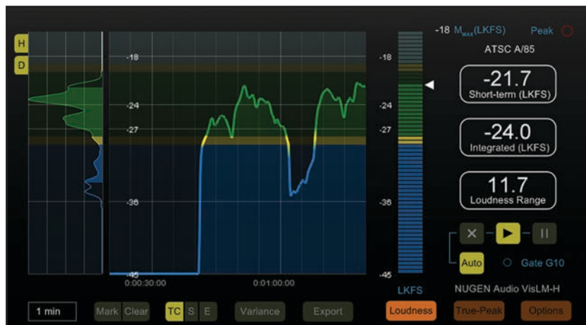
The NUGEN Audio VisLM loudness meter shows S_{MAX}-M_{MAX} toggles and history color bands to highlight loudness boundaries.
