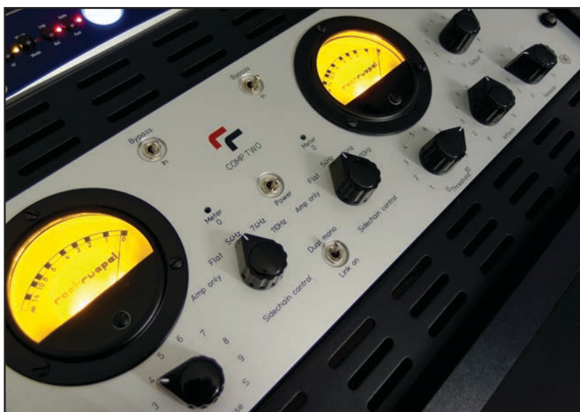
The Rockruepel comp.two is an all-tube hand-built stereo compressor made in Germany. This comp.one successor is a more refined and straightforward unit.
