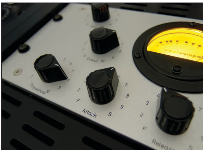
The comp.two's front panel seems like a standard variable- \mu compressor with input, output, threshold, and attack and release settings. This unit also features Hoyt volume unit (VU) meters.
