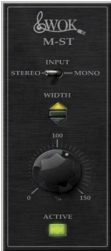
Photo 2: As with the Widebug, the M-ST input and output levels must be set in the host. Although it accepts a mono input, this does not produce a stereo output file and the expansion is limited to just 150%.
