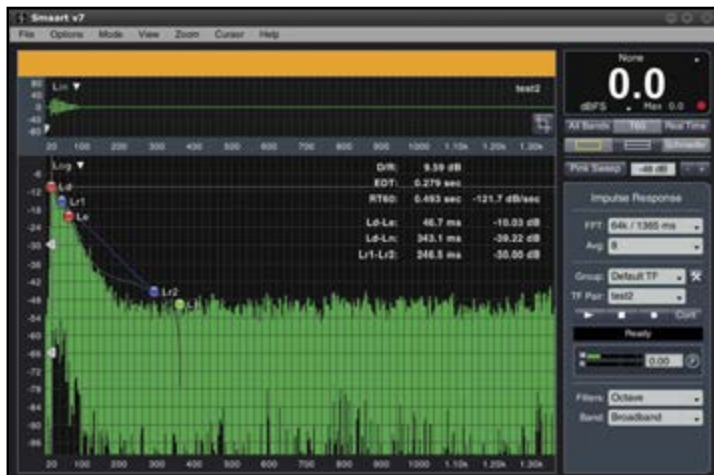
Photo 7: The RT60 decay can be displayed for a chosen octave or 1/3-octave band.
