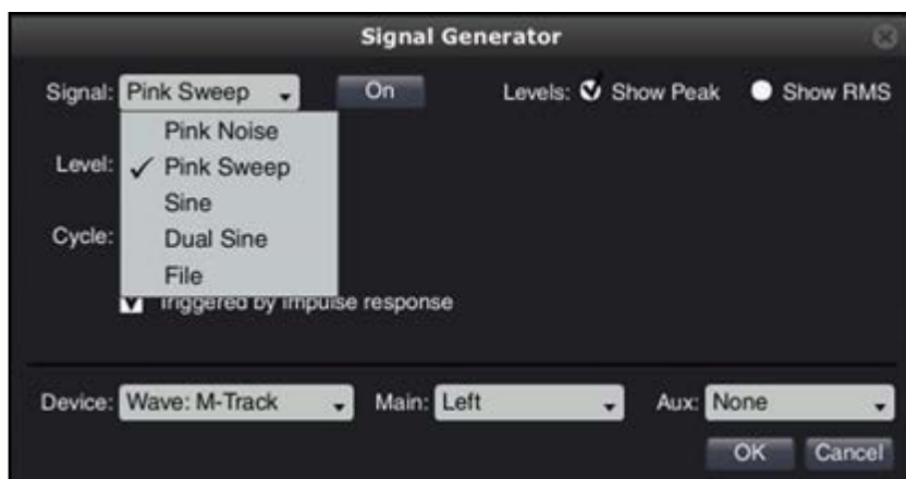
Photo 4: The signal generator control panel enables selection of signal-source parameters.
