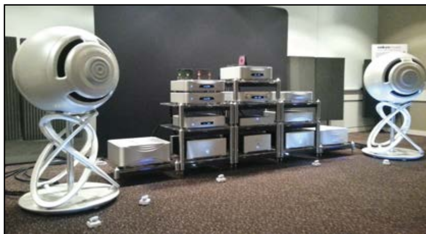
Photo 16: Living large—Cabasse's new La Sphère is a grander version of the L'Océan, and employs a generous 22" honeycomb dome woofer behind a triaxial 1.1" polyether tweeter, 4" P2C annular mid, and an 8" Duocell annular low-mid.
