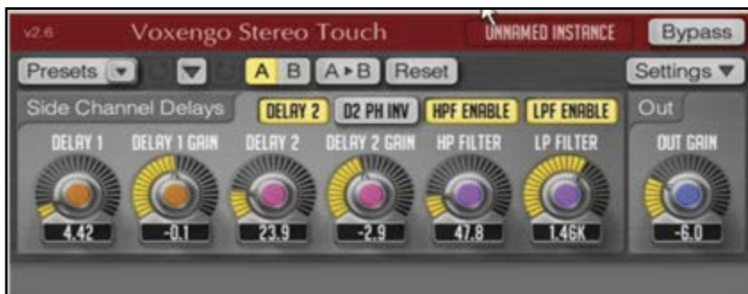
Photo 3: The Stereo Touch interface looks complex but several presets are included and you can easily make changes to them to observe the effect on the expansion.
