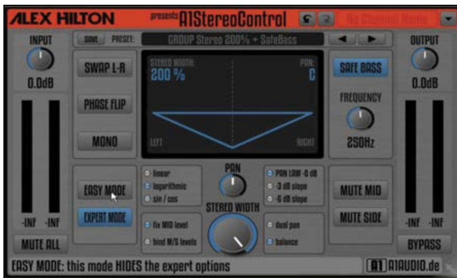
Photo 4: Alex Hilton did an excellent job designing this free plug-in. His SafeBass option correctly puts the low frequencies in the soundstage center. There are several presets to get you started.
