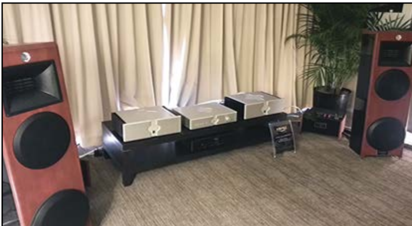
Photo 13: The supertweeter-equipped Soundfield Audio Dipole 1 has a semi-active, open-baffle design.
