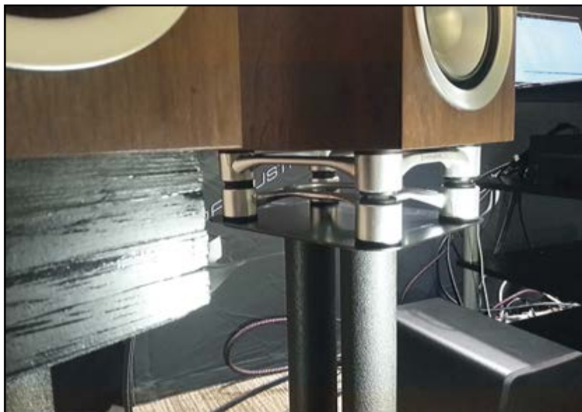
Photo 9: The proof is in the listening—wood blocks vs. IsoAcoustics' new Aperta isolation mounts.
