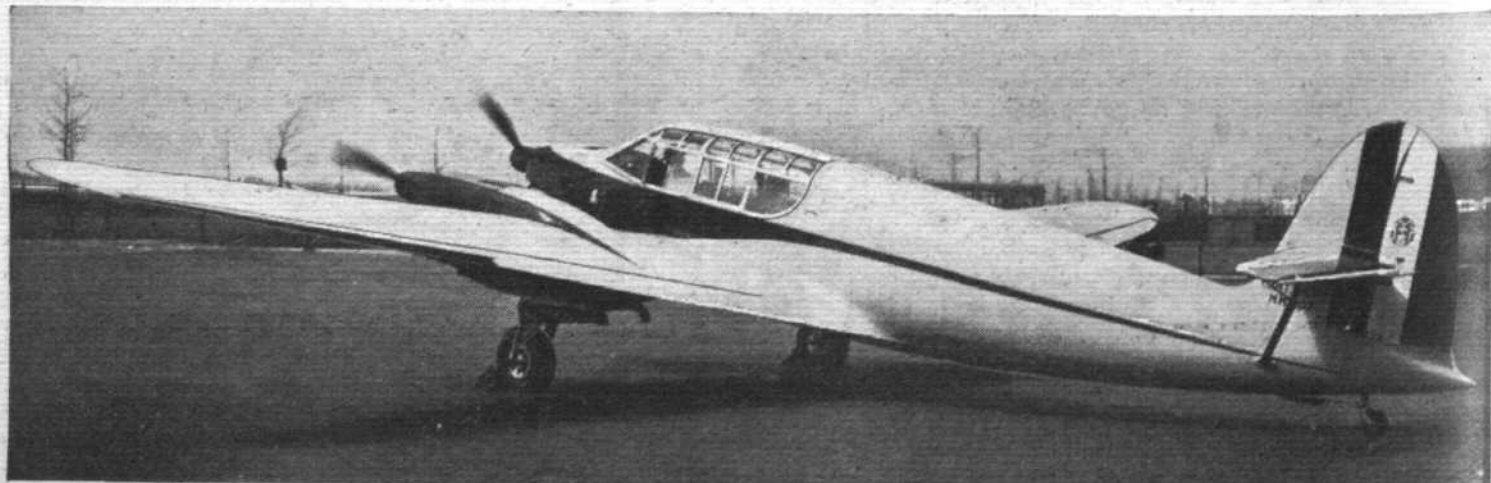
ATTACHED: Imported for the use of Col. Vincenzo Coppola, the Air and Military Attaché to the Italian Embassy in Washington, this Cant monoplaner has three 110 h.p. inverted four-cylinder Fiat engines. It was assembled at the Floyd Bennet Field.
