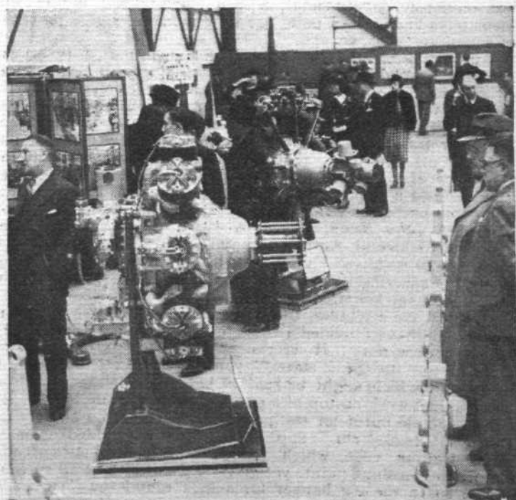
Power quiescent: Bristol engines in the "static" show, with a sleeve-valve Aquila in the foreground.
