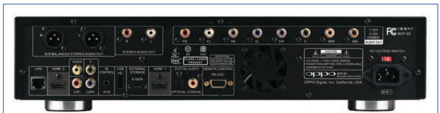
Photo 2: Rear panel of the BDP-95. The player offers the same digital and video connectivity as the BDP-93, but the audio portion includes dedicated two-channel outputs for the highest possible performance from stereo material. (Photo courtesy of Oppo Digital)
