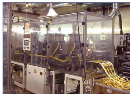
Photo 2: Automated spider manufacturing at Loudspeaker Components Corporation's facility in Nogales, Mexico
