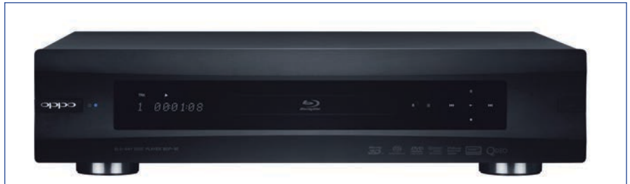
Photo 1: The front panel of the BDP-95 Universal Blu-ray player is extremely attractive. A touch-sensitive array on the right side of the display controls basic transport functions. Power and Eject buttons are mounted flush with the front panel. (Photo courtesy of Oppo Digital)
