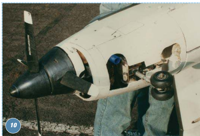
7 & 8: The triple-cockpit upper fuselage panel is made removable for access to the radio equipment bay. 9: Main undercarriage leg and wheel well. There is no rake-forward/rake-back 'double angle' geometry to contend with in arranging undercarriage retraction. 10: The retracting noseleg unit installation. Note also the simulated contra-rotation propellers, the dummy component being the rear pair of blades, set in the 'feathered' position, often operated in that state on the full size aircraft for cruise economy while on patrol.
