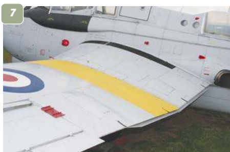
4: Aileron underside on the wing of Midland Air Museum's Gannet T.2. 5: Aileron upper surface, also showing square raised blister inboard. 6: Wing outer panel underside, showing weapons rails. 7: Wing upper surface detail on T.2, showing wing walk pad. 8: Wing outer panel showing leading edge and wing trip lights. 9: Retracted flap panel. 10 & 11: Contra-rotating propeller unit is a prominent feature of the Gannet. 12: Bird or Basking Shark? The gaping front end of the Gannet that ducts airflow to the Double Mamba engine. 13: Further nose section detail. Note the periscope atop the cockpit (T.2 variant). 14: Nosewheel door detail. The main (rear) doors on 'working' Gannets actually closed after the leg was extended.
