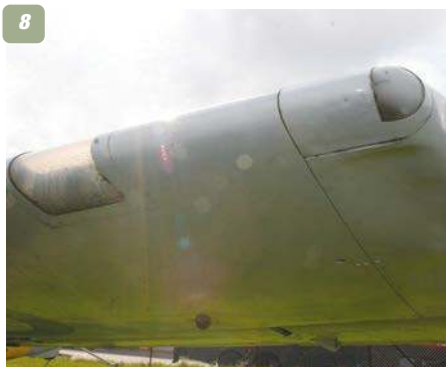
4: Aileron underside on the wing of Midland Air Museum's Gannet T.2. 5: Aileron upper surface, also showing square raised blister inboard. 6: Wing outer panel underside, showing weapons rails. 7: Wing upper surface detail on T.2, showing wing walk pad. 8: Wing outer panel showing leading edge and wing trip lights. 9: Retracted flap panel. 10 & 11: Contra-rotating propeller unit is a prominent feature of the Gannet. 12: Bird or Basking Shark? The gaping front end of the Gannet that ducts airflow to the Double Mamba engine. 13: Further nose section detail. Note the periscope atop the cockpit (T.2 variant). 14: Nosewheel door detail. The main (rear) doors on 'working' Gannets actually closed after the leg was extended.
