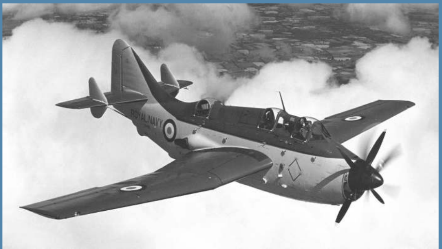
A Gannet AS Mk.4, with the rear element of the contra-prop unit fully feathered.
