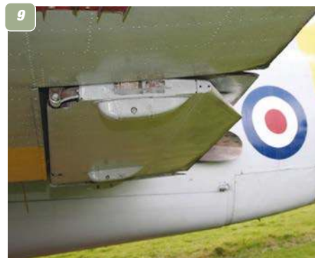
4: Aileron underside on the wing of Midland Air Museum's Gannet T.2. 5: Aileron upper surface, also showing square raised blister inboard. 6: Wing outer panel underside, showing weapons rails. 7: Wing upper surface detail on T.2, showing wing walk pad. 8: Wing outer panel showing leading edge and wing trip lights. 9: Retracted flap panel. 10 & 11: Contra-rotating propeller unit is a prominent feature of the Gannet. 12: Bird or Basking Shark? The gaping front end of the Gannet that ducts airflow to the Double Mamba engine. 13: Further nose section detail. Note the periscope atop the cockpit (T.2 variant). 14: Nosewheel door detail. The main (rear) doors on 'working' Gannets actually closed after the leg was extended.
