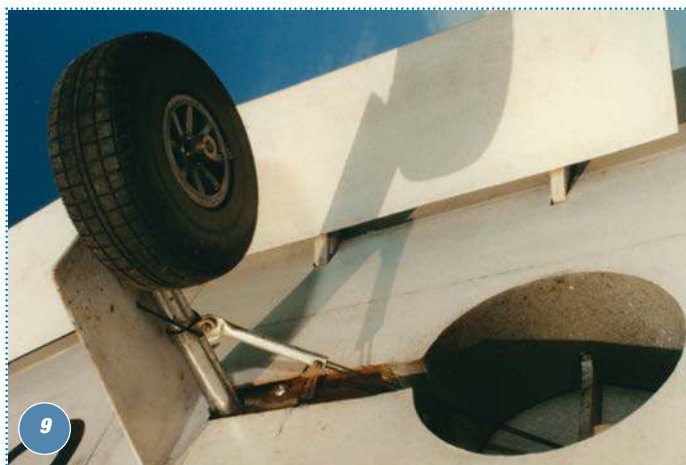
7 & 8: The triple-cockpit upper fuselage panel is made removable for access to the radio equipment bay. 9: Main undercarriage leg and wheel well. There is no rake-forward/rake-back 'double angle' geometry to contend with in arranging undercarriage retraction. 10: The retracting noseleg unit installation. Note also the simulated contra-rotation propellers, the dummy component being the rear pair of blades, set in the 'feathered' position, often operated in that state on the full size aircraft for cruise economy while on patrol.
