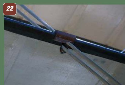
18: View inside the access hatch in the left fuselage side just behind the engine cowling. 19: Anchor point on the fin for the rear streamline brace between the fin and tailplane upper surface. 20: Anchor point on the fin leading edge for the front brace between fin and tailplane upper surface. 21: Fin, and tailplane upper surface, showing braces and elevator control horn. 22: Double streamline braces that link the fuselage and upper wing, showing how it passes through the centre wing leading edge. 23: The bottom anchor point on the lower fuselage side for those same bracing wires. 24: Brace anchor points on the upper wing underside. 25: Detail of bracing wire that runs from the rear of the engine cowl to the wing leading edge. 26: Anchor point for brace in the bottom wing upper surface at the wing root, at about mid-chord. 27: Attachment point on the centre wing aileron upper surface for wire linking the three ailerons. 28: Step in the left bottom fuselage side, just behind the wing for access to the cockpit. Note also the 'eared' nut to the left of the step ... what you might call a true wing nut! 29: The electric generator, facing rearwards, mounted on the right hand centre section strut between the centre and upper wings. 30: View of the tailplane leading edge showing elevator control runs and bracing wires. 31: Front tailplane bracing wire anchor point on the upper surface.
