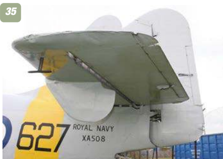
29: The arrestor hook looks quite spindly to stop an aircraft as big as the Gannet! 30: Detail of the hook end. 31: Detail of the rudder hinge-line. 32: Anchor point for the arrestor hook shaft and the tail bumper. 33 & 34: Exhaust effluxes of the Armstrong Siddeley Double Mamba engine, just behind the wing trailing edges, left and right. 35: Tailplane/elevator hinge line detail on Midland A.M.'s Gannet T.2 also reveals the auxilliary underside fin and rather mangled tailplane tip! 36: Auxilliary fin on the tailplane upper surface. 37: Side view of one for the nosewheels. 38: Twin nosewheels, viewed from the rear.
