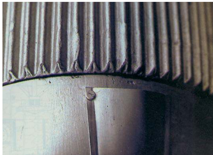
Detail of corrugation edge crimping, here at the engine firewall.
