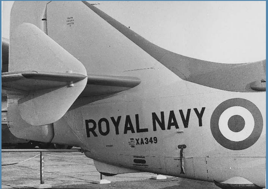
A Gannet AS Mk.4, rear showing the auxiliary fins applied to the tailplane.
