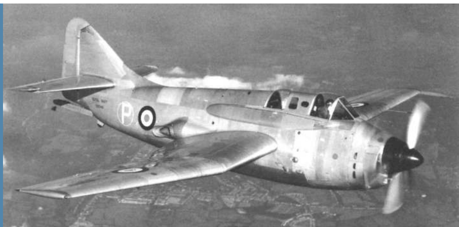
The first prototype, the Fairey Q, the interim designated Fairey Type 17, showing the original two-seat crew configuration.
