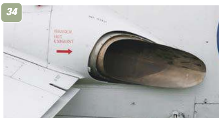
29: The arrestor hook looks quite spindly to stop an aircraft as big as the Gannet! 30: Detail of the hook end. 31: Detail of the rudder hinge-line. 32: Anchor point for the arrestor hook shaft and the tail bumper. 33 & 34: Exhaust effluxes of the Armstrong Siddeley Double Mamba engine, just behind the wing trailing edges, left and right. 35: Tailplane/elevator hinge line detail on Midland A.M.'s Gannet T.2 also reveals the auxilliary underside fin and rather mangled tailplane tip! 36: Auxilliary fin on the tailplane upper surface. 37: Side view of one for the nosewheels. 38: Twin nosewheels, viewed from the rear.
