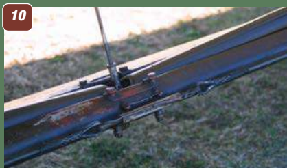
9: View of the undercarriage cross-member viewed from above, showing the associated bracing wires. 10: Close-up of the bracing wire centre anchor point on the main undercarriage cross member. 11: Anchor point for the front main undercarriage leg, just behind the engine cowl. 12: General layout of the main undercarriage. 13 & 14: Two views inside the cockpit. 15, 16 & 17: Three views of the engine cowl, showing the rotary engine and the slots in the bottom of the cowl.
