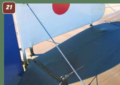
18: View inside the access hatch in the left fuselage side just behind the engine cowling. 19: Anchor point on the fin for the rear streamline brace between the fin and tailplane upper surface. 20: Anchor point on the fin leading edge for the front brace between fin and tailplane upper surface. 21: Fin, and tailplane upper surface, showing braces and elevator control horn. 22: Double streamline braces that link the fuselage and upper wing, showing how it passes through the centre wing leading edge. 23: The bottom anchor point on the lower fuselage side for those same bracing wires. 24: Brace anchor points on the upper wing underside. 25: Detail of bracing wire that runs from the rear of the engine cowl to the wing leading edge. 26: Anchor point for brace in the bottom wing upper surface at the wing root, at about mid-chord. 27: Attachment point on the centre wing aileron upper surface for wire linking the three ailerons. 28: Step in the left bottom fuselage side, just behind the wing for access to the cockpit. Note also the 'eared' nut to the left of the step ... what you might call a true wing nut! 29: The electric generator, facing rearwards, mounted on the right hand centre section strut between the centre and upper wings. 30: View of the tailplane leading edge showing elevator control runs and bracing wires. 31: Front tailplane bracing wire anchor point on the upper surface.
