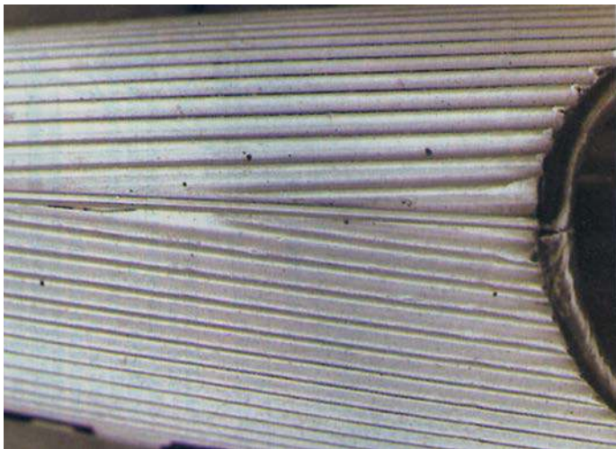
Join line of corrugated sheet along the top of the fuselage centre line. Underside is similar.
