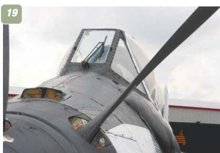
15: Radar operator's rear cockpit bubble. 16: Detail of the two forward cockpits. Note the periscope (Gannet T.2) and the wing walk pads. 17: All three cockpits, showing the distinctive bulged strake under the cockpit sills. 18: The driving seat, pilot's position. 19: View over the nose, showing the cockpit windscreen wiper. 20: Another view of the two front cockpits, seen from the left side. 21 & 22: The line of the bomb bay. Note also the folding step ladder. 23: Massive hook under the wing leading edge engages the catapult-launch 'strop'. 24-28: Views of the massive main undercarriage.
