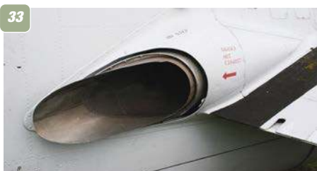
29: The arrestor hook looks quite spindly to stop an aircraft as big as the Gannet! 30: Detail of the hook end. 31: Detail of the rudder hinge-line. 32: Anchor point for the arrestor hook shaft and the tail bumper. 33 & 34: Exhaust effluxes of the Armstrong Siddeley Double Mamba engine, just behind the wing trailing edges, left and right. 35: Tailplane/elevator hinge line detail on Midland A.M.'s Gannet T.2 also reveals the auxilliary underside fin and rather mangled tailplane tip! 36: Auxilliary fin on the tailplane upper surface. 37: Side view of one for the nosewheels. 38: Twin nosewheels, viewed from the rear.
