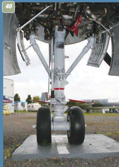
39: The tall noseleg gives the Gannet a distinct tail-down sit. 40: A further view of the noseleg unit, viewed from the rear.
