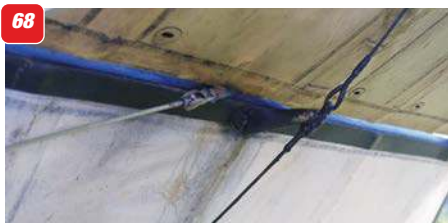
67 & 68: Underside of tailplane and elevator, showing bracing wires and clear vision inspection panel. 69: Wing entire section inspection panel on Shuttleworth machine, non-standard. 70: Lower left wing centre section showing tread plates and bracing wire anchors. 71: Close up of rear tread plate at wing root. Note also the release tab for the wing panel. 72: Wing panel release tab on lower wing root underside. 73: Aileron, showing hinge line. 74: Lower centre section front tread plate and brace wire anchor point 75: Upper wing centre section showing the overflow pipes and the faired attachment points for the Lewis gun rail. 76: Clear vision panel, upper wing tip underside. 77 & 78: The steerable tail skid, also showing the bracing wires to the tailplane underside and the steering horn for the tailskid. 79: Lower wing underside, showing the aileron and the control horn.
