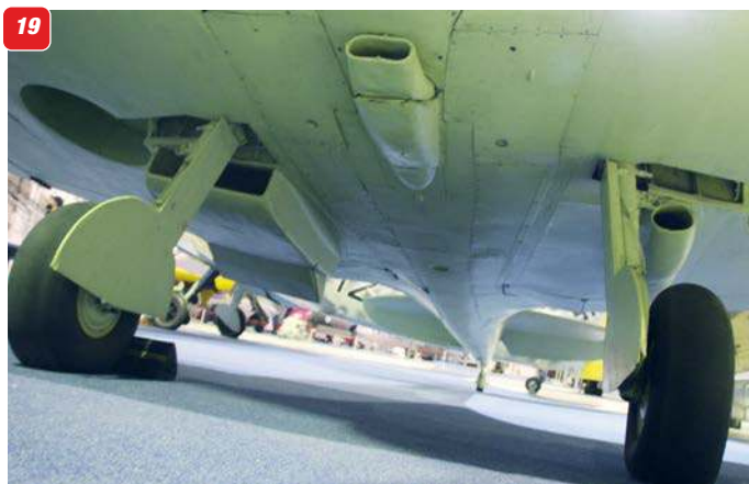
16 & 17: Two views of the main undercarriage wells. Note the stiffeners. 18: Wing underside, showing access panels to the guns and the spent rounds exits. 19: Rearward view of the fuselage/wingroot underside. Note the "gull" shape of the fairing panel at the wing trailing edge. 20: Fin and rudder. Tapes and stitching to the fabric of the rudder are prominent, also seen in 21 . 22: The rudder trim tab and drive, right side only. 23: Carburettor air intake, placed at the wing/fuselage underside centre line. 25 & 26: The radiator, right wing underside. 27: Further view of the radiator, from the rear. Note also the prominent "gull" shape of the wing-to-fuselage fairing trailing edge.
