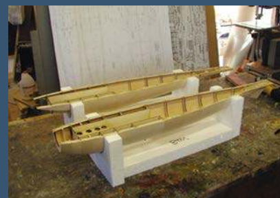
This sequence is a good example of a rounded fuselage built as two half-shells, top and bottom, in which the balsa surface skin is applied to each of the shells before joining. The aircraft being modelled here is the Albatros D5a late WW1 fighter type.
