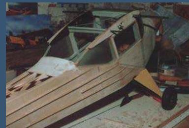
This Auster J/5 Adventurer is an example of the not-quite-flat-sided rear fuselage shape in which fore/aft stringers have been applied over the flat balsa sheet sides to get to the right, scale, fuselage section.
