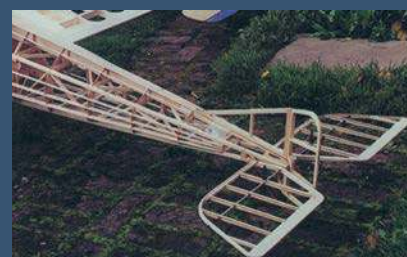
The early WW1-era Moraine Saulnier Type N fighter/scout was an early attempt at a streamlined fuselage. Illustrated here is a finished airframe in which a basic square box is rounded to profile with circular sub-formers applied around the box structure uprights.
