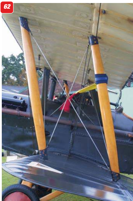
55: Front strut attachment under upper wing. 56: Rear strut anchor point under upper wing. 57: Centre section (cabane) struts. 58: Rear interplane strut anchor on lower wing. 59: Similar for front strut. 60: Pitot head. 61: The right side cabane struts. 62: General arrangement of interplane struts.
