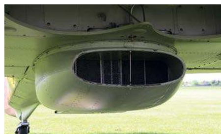
The Hawker Hurricane had one large fuselage-mounted radiator installed on the centreline on the wing underside. Front and rear views here illustrate the front intake and the rear air outlet. Doubtful if the rather small centreline carburettor intake scoop, forward of the radiator, would be worth adapting for cooling purpose. Much effort for little gain!
