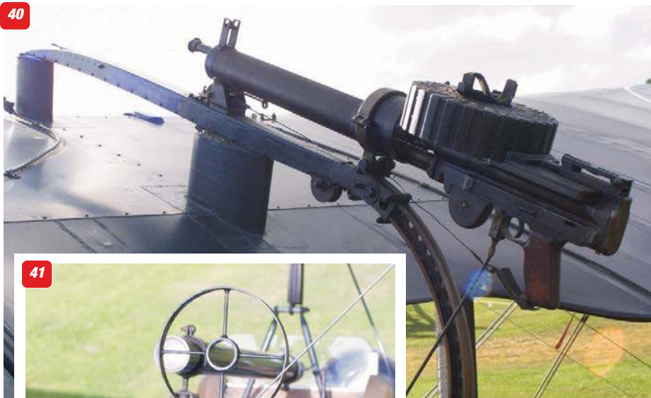
37: Tailpost, viewed from under the tailplane 38: The Lewis gun installation - gun slides back and down on curved rail. 39: The gun sight tube, showing front mounting and panels. 40: The rail for the Lewis gun mounting is secured to the upper wind centre section by two faired mounting blocks. 41: Business end of the left fuselage mounted 0.303" calibre Lewis, fixed-mounted under fairing. Also shows the ring sight and chamber mounted ring sight.
