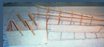
The early WW1-era Moraine Saulnier Type N fighter/scout was an early attempt at a streamlined fuselage. Illustrated here is a finished airframe in which a basic square box is rounded to profile with circular sub-formers applied around the box structure uprights.
