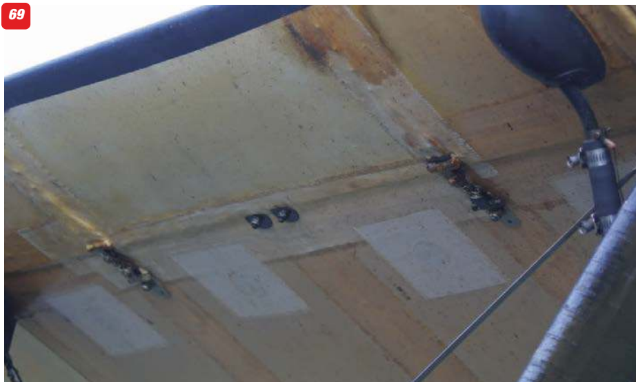
67 & 68: Underside of tailplane and elevator, showing bracing wires and clear vision inspection panel. 69: Wing entire section inspection panel on Shuttleworth machine, non-standard. 70: Lower left wing centre section showing tread plates and bracing wire anchors. 71: Close up of rear tread plate at wing root. Note also the release tab for the wing panel. 72: Wing panel release tab on lower wing root underside. 73: Aileron, showing hinge line. 74: Lower centre section front tread plate and brace wire anchor point 75: Upper wing centre section showing the overflow pipes and the faired attachment points for the Lewis gun rail. 76: Clear vision panel, upper wing tip underside. 77 & 78: The steerable tail skid, also showing the bracing wires to the tailplane underside and the steering horn for the tailskid. 79: Lower wing underside, showing the aileron and the control horn.
