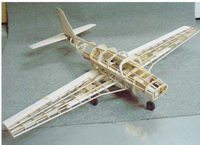
Dave Gamblin's delightful electric powered Piper Comanche features both planked and sheeted covering over a light framework.
