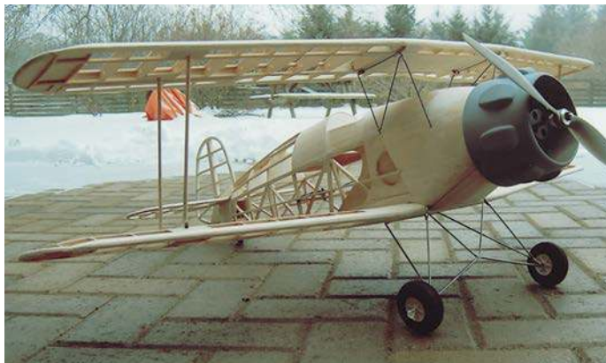
Chris McHugh's Bucker Jungmeister displays a typical lightweight biplane fuselage structure with open-frame rear.
