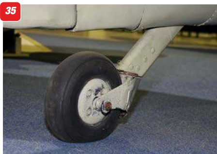
34 & 35: Two views of the non-retractable, castoring tailwheel.
