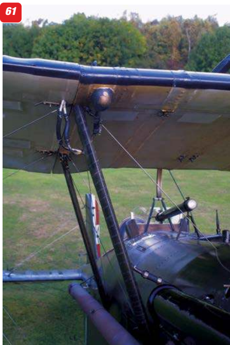
55: Front strut attachment under upper wing. 56: Rear strut anchor point under upper wing. 57: Centre section (cabane) struts. 58: Rear interplane strut anchor on lower wing. 59: Similar for front strut. 60: Pitot head. 61: The right side cabane struts. 62: General arrangement of interplane struts.
