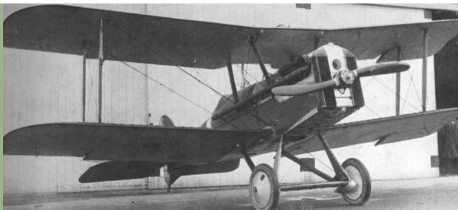
An early Wolsey Viper engine installation on an S.E.5. The top of the radiator differs from the shape that became standard, while the nose section underfiring is more shallow than on Viper powered production aircraft.
