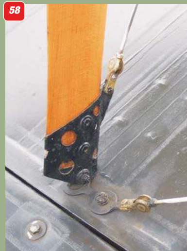
55: Front strut attachment under upper wing. 56: Rear strut anchor point under upper wing. 57: Centre section (cabane) struts. 58: Rear interplane strut anchor on lower wing. 59: Similar for front strut. 60: Pitot head. 61: The right side cabane struts. 62: General arrangement of interplane struts.
