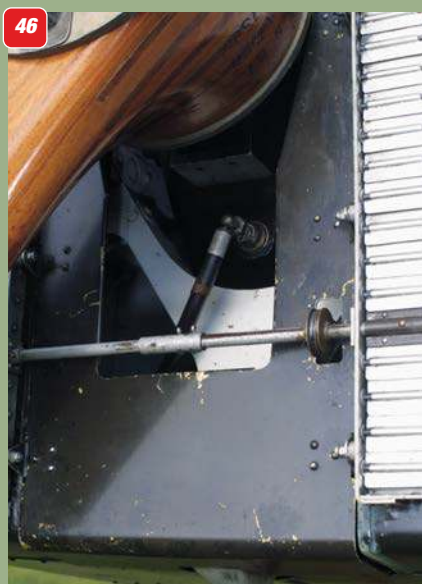
42 & 43: Two views of the cockpit windscreen. Note also the anchor bracket to the Lewis gun rail. 44-47: The radiator and propeller hub. Note that 46 shows the pulley type control to the radiator shutters. 48: Upper engine cowling, with air gaps between panels. 49: Radiator filler cap. Note the lack of fit between the radiator rear and the front of the cowl panel behind it. 50: Anchor point for bracing wires at lower fuselage, just above rear undercarriage attachment. 51 & 52: Fuel line from emergency tank in wing centre section. Note cabane strut binding. 53: Cabane strut attachment to wing upper centre section. 54: Flying wire anchor, under upper wing.
