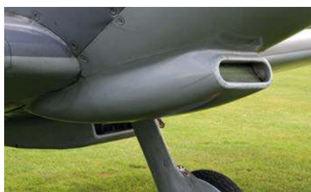
From the Mk.IX onward, Supermarine Spitfires had two large radiators mounted one under each wing which could be used as air scoops/ warm air outlet ducts as illustrated in Fig.1. The centrally mounted nose underside mounted carburettor air intake can also be used for air ducting.
