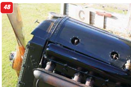
42 & 43: Two views of the cockpit windscreen. Note also the anchor bracket to the Lewis gun rail. 44-47: The radiator and propeller hub. Note that 46 shows the pulley type control to the radiator shutters. 48: Upper engine cowling, with air gaps between panels. 49: Radiator filler cap. Note the lack of fit between the radiator rear and the front of the cowl panel behind it. 50: Anchor point for bracing wires at lower fuselage, just above rear undercarriage attachment. 51 & 52: Fuel line from emergency tank in wing centre section. Note cabane strut binding. 53: Cabane strut attachment to wing upper centre section. 54: Flying wire anchor, under upper wing.
