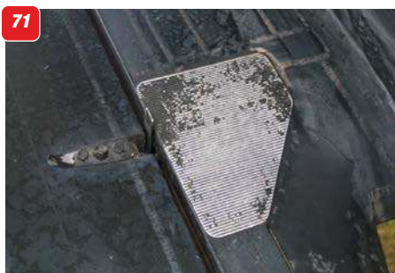
67 & 68: Underside of tailplane and elevator, showing bracing wires and clear vision inspection panel. 69: Wing entire section inspection panel on Shuttleworth machine, non-standard. 70: Lower left wing centre section showing tread plates and bracing wire anchors. 71: Close up of rear tread plate at wing root. Note also the release tab for the wing panel. 72: Wing panel release tab on lower wing root underside. 73: Aileron, showing hinge line. 74: Lower centre section front tread plate and brace wire anchor point 75: Upper wing centre section showing the overflow pipes and the faired attachment points for the Lewis gun rail. 76: Clear vision panel, upper wing tip underside. 77 & 78: The steerable tail skid, also showing the bracing wires to the tailplane underside and the steering horn for the tailskid. 79: Lower wing underside, showing the aileron and the control horn.
