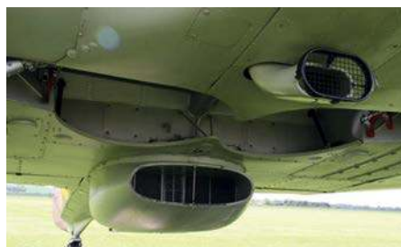
The Hawker Hurricane had one large fuselage-mounted radiator installed on the centreline on the wing underside. Front and rear views here illustrate the front intake and the rear air outlet. Doubtful if the rather small centreline carburettor intake scoop, forward of the radiator, would be worth adapting for cooling purpose. Much effort for little gain!
