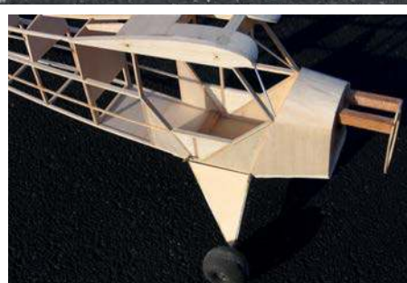
The Piper J-3 Cub fuselage rear section is close to, but not quite flat sided, in which side stringers are applied to the upright spacers of the open box structure to achieve the true-scale fuselage cross section
