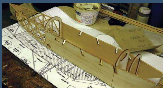
The Westland Widgeon III is an example of the 'basic-box-plus-rounded-top-deck. In this example the rear, open-frame structure is built separately from the balsa sheet, flat-sided assembly.
