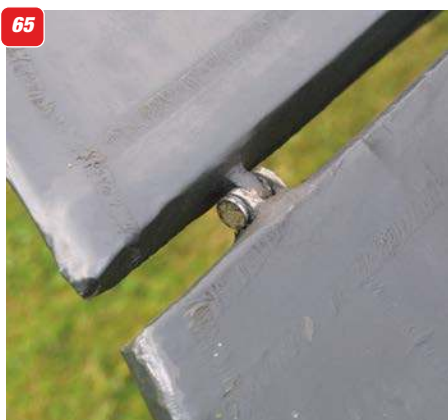
63: Anchor points for tailplane bracing. Note clear vision inspection panel to aileron cable pulley. 64: Elevator control wire run to elevator horn also showing clear inspection panel. 65: Simple metal elevator hinge. 66: Elevator horn.
