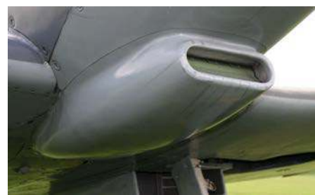
From the Mk.IX onward, Supermarine Spitfires had two large radiators mounted one under each wing which could be used as air scoops/ warm air outlet ducts as illustrated in Fig.1. The centrally mounted nose underside mounted carburettor air intake can also be used for air ducting.
