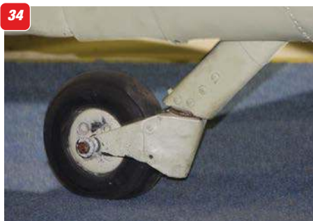
34 & 35: Two views of the non-retractable, castoring tailwheel.
