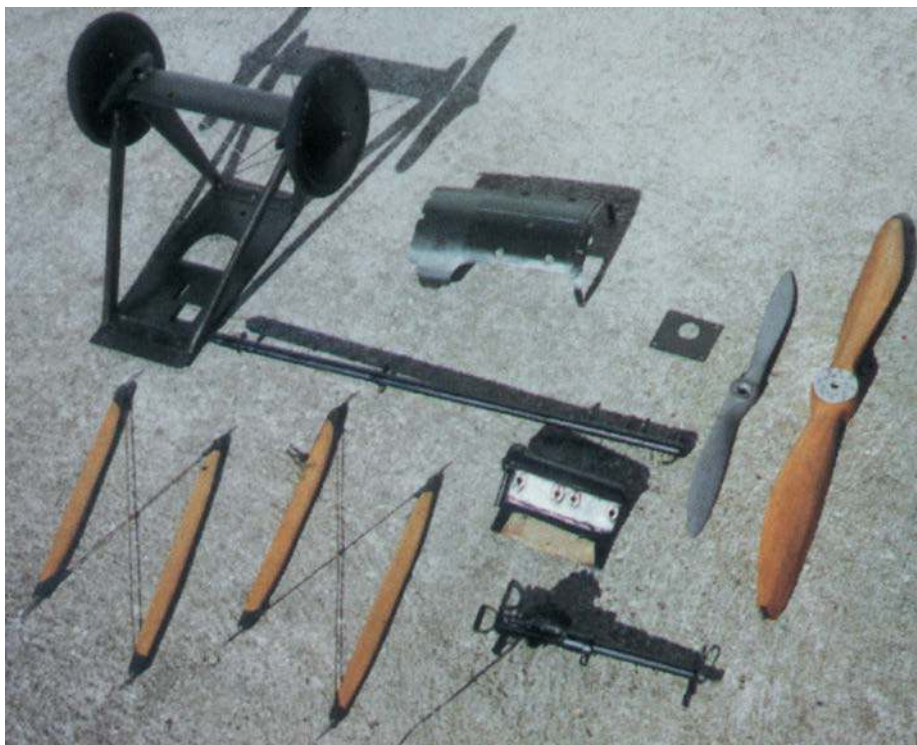
Gary's dismantled prototype model reveals the individual component parts, and provides a good idea of how it assembled. The interplane struts have wire pegs top and bottom to locate into the upper surfaces of the lower wings, and lower surfaces of the top wings. Note the static display scale propeller.
