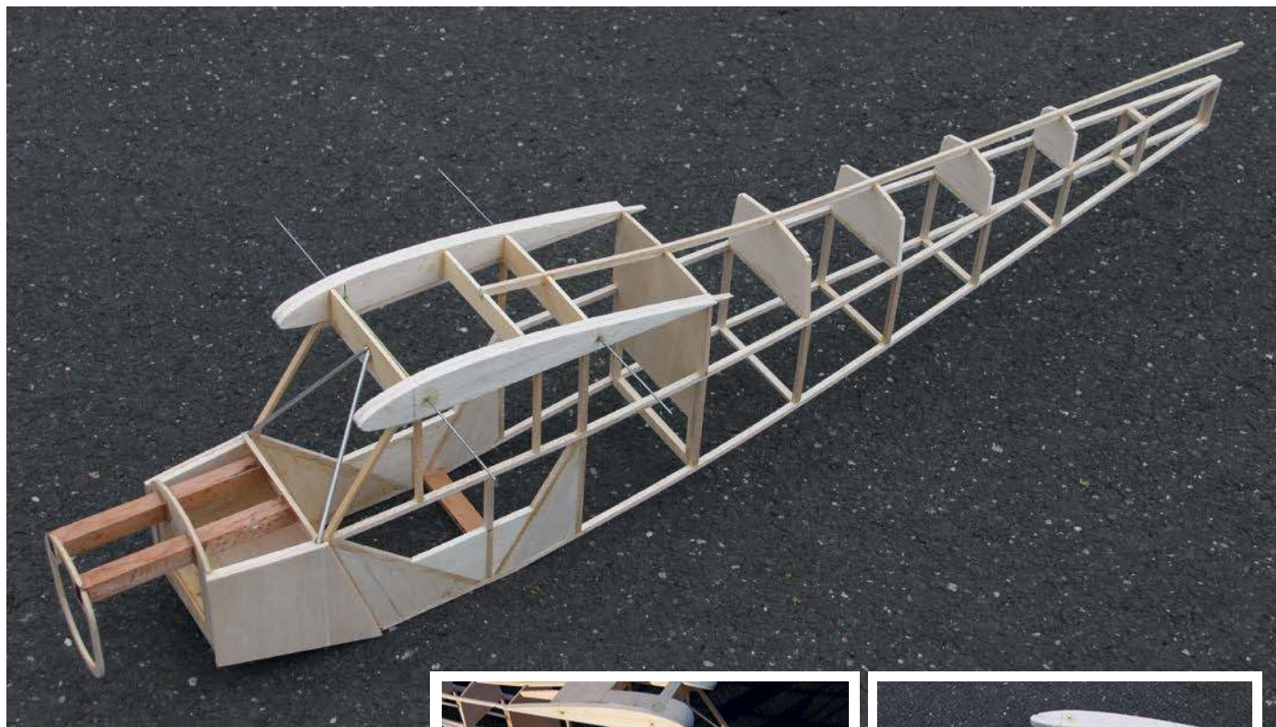
The Piper J-3 Cub fuselage rear section is close to, but not quite flat sided, in which side stringers are applied to the upright spacers of the open box structure to achieve the true-scale fuselage cross section
