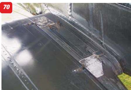
67 & 68: Underside of tailplane and elevator, showing bracing wires and clear vision inspection panel. 69: Wing entire section inspection panel on Shuttleworth machine, non-standard. 70: Lower left wing centre section showing tread plates and bracing wire anchors. 71: Close up of rear tread plate at wing root. Note also the release tab for the wing panel. 72: Wing panel release tab on lower wing root underside. 73: Aileron, showing hinge line. 74: Lower centre section front tread plate and brace wire anchor point 75: Upper wing centre section showing the overflow pipes and the faired attachment points for the Lewis gun rail. 76: Clear vision panel, upper wing tip underside. 77 & 78: The steerable tail skid, also showing the bracing wires to the tailplane underside and the steering horn for the tailskid. 79: Lower wing underside, showing the aileron and the control horn.
