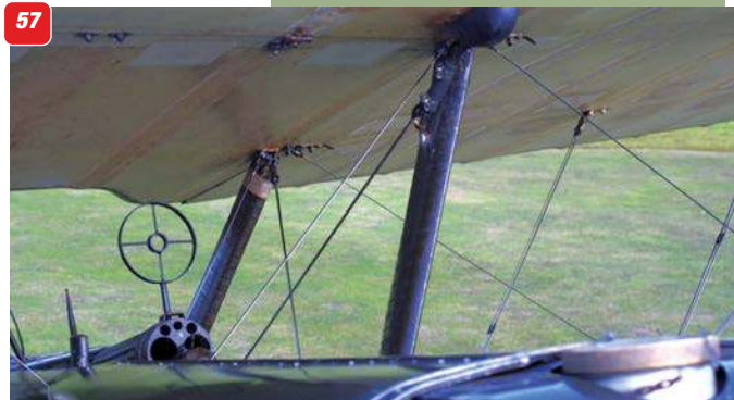
55: Front strut attachment under upper wing. 56: Rear strut anchor point under upper wing. 57: Centre section (cabane) struts. 58: Rear interplane strut anchor on lower wing. 59: Similar for front strut. 60: Pitot head. 61: The right side cabane struts. 62: General arrangement of interplane struts.
