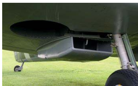
From the Mk.IX onward, Supermarine Spitfires had two large radiators mounted one under each wing which could be used as air scoops/ warm air outlet ducts as illustrated in Fig.1. The centrally mounted nose underside mounted carburettor air intake can also be used for air ducting.
