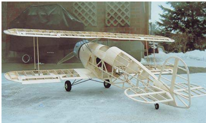
Chris McHugh's Bucker Jungmeister displays a typical lightweight biplane fuselage structure with open-frame rear.
