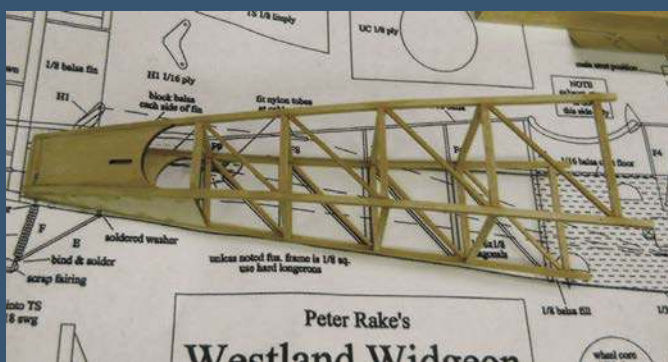
The Westland Widgeon III is an example of the 'basic-box-plus-rounded-top-deck. In this example the rear, open-frame structure is built separately from the balsa sheet, flat-sided assembly.
