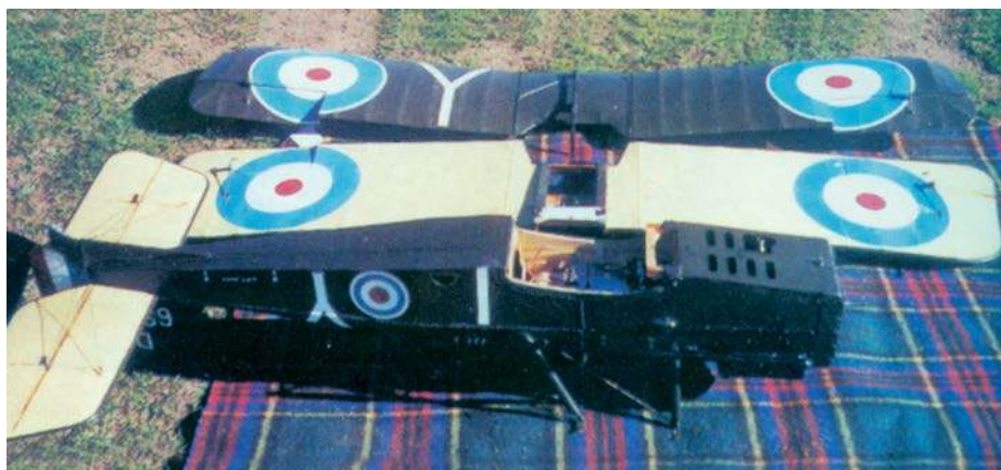
At 1/5th scale there is really no need for separate left and right wing panels and the model will easily fit into a modestly sized vehicle for transport. Assembly is therefore quick.
