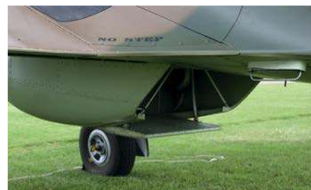
The Hawker Hurricane had one large fuselage-mounted radiator installed on the centreline on the wing underside. Front and rear views here illustrate the front intake and the rear air outlet. Doubtful if the rather small centreline carburettor intake scoop, forward of the radiator, would be worth adapting for cooling purpose. Much effort for little gain!
