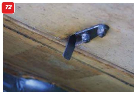
67 & 68: Underside of tailplane and elevator, showing bracing wires and clear vision inspection panel. 69: Wing entire section inspection panel on Shuttleworth machine, non-standard. 70: Lower left wing centre section showing tread plates and bracing wire anchors. 71: Close up of rear tread plate at wing root. Note also the release tab for the wing panel. 72: Wing panel release tab on lower wing root underside. 73: Aileron, showing hinge line. 74: Lower centre section front tread plate and brace wire anchor point 75: Upper wing centre section showing the overflow pipes and the faired attachment points for the Lewis gun rail. 76: Clear vision panel, upper wing tip underside. 77 & 78: The steerable tail skid, also showing the bracing wires to the tailplane underside and the steering horn for the tailskid. 79: Lower wing underside, showing the aileron and the control horn.
