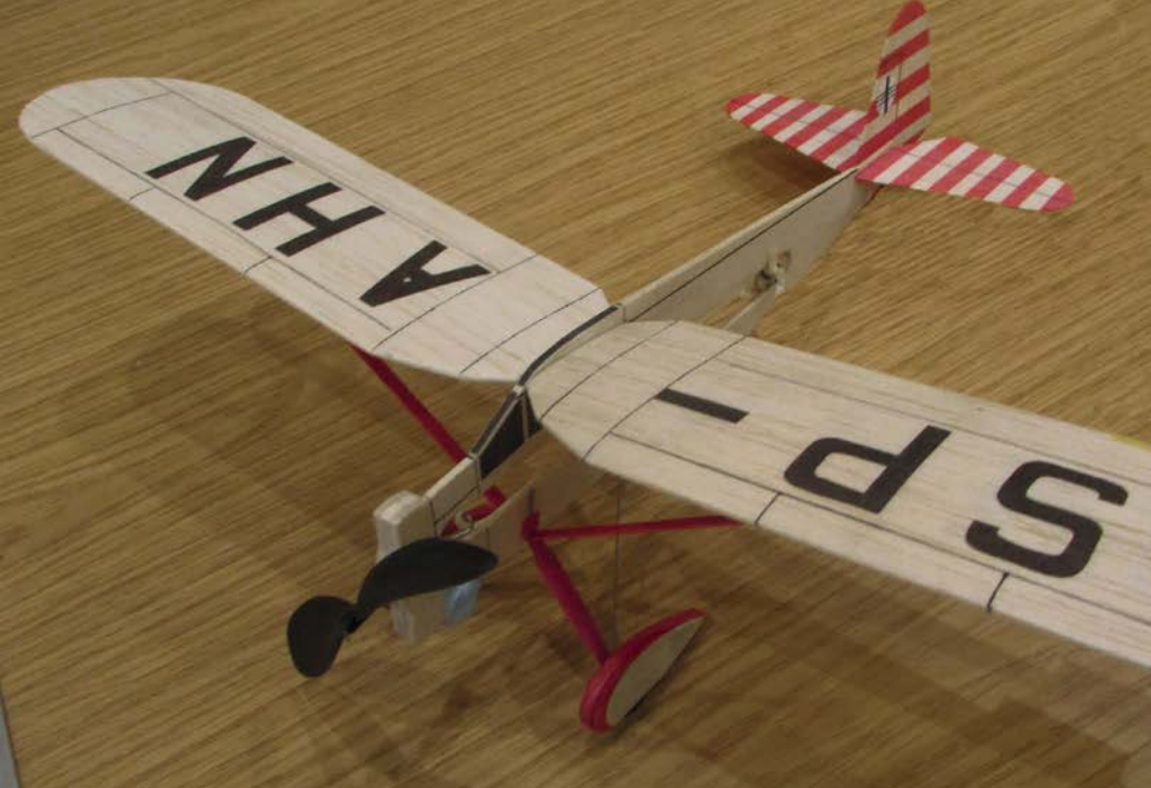
A fun model slabsider from John Slate of the Polish RWD6 with a single loop of rubber and 1,200 turns.
