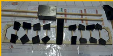
Covering the plan with thin, clear polythene/plastic ensures the glue does not stick your tailplane to the plan. Sensible use of weights and pins while the glue dries will result in a flat and robust structure.
