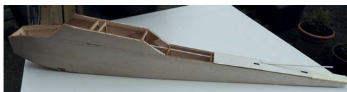
It is easiest to fit the control runs (Bowden/snake outers) before completing the top and sheeting.
