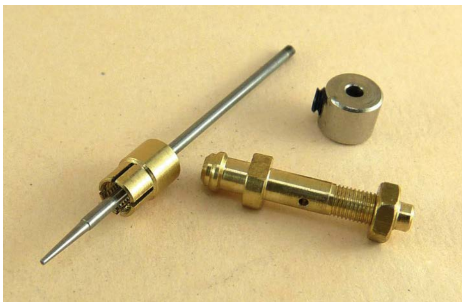
Needle valve assembly provides excellent fuel metering. Owner determines where to bend elbow and final length of needle extension. Or add a wheel collar to form an adjusting knob.
