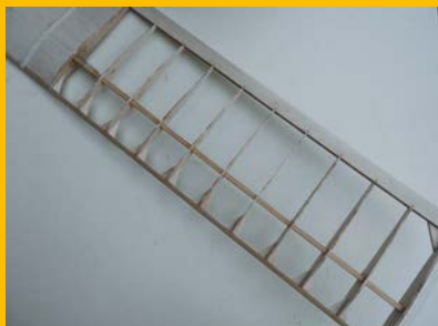
The Trailing Edge is nicely indented by laser cutting for the rib ends. Ann decided to take a 'belt and braces' approach to strengthen the LE by adding gussets – not strictly necessary but good on a training model which will get additional knocks.
