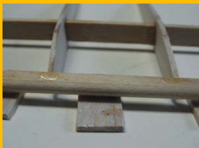
Ann found that it helped to pack the LE strip up with scrap balsa when fitting and gluing it to the ribs.
