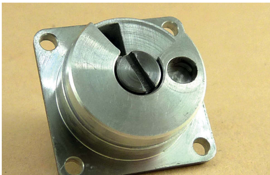
Barely perceptible circular "witness marks" after extensive testing suggest the disc/rotor and back plate will not suffer undue wear in service, providing dirt is excluded. Assembly could be repositioned 90 degrees clockwise (viewed from rear) for running in reverse direction. That would point needle downwards (or upright if cylinder is inverted).
