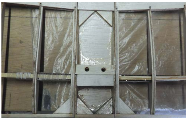
The left and right wing panels are glued in place propped to the correct dihedral while the centre section is held flat on the work bench. Once the glue is dry then the dihedral brace is bound to the main wing spar.
