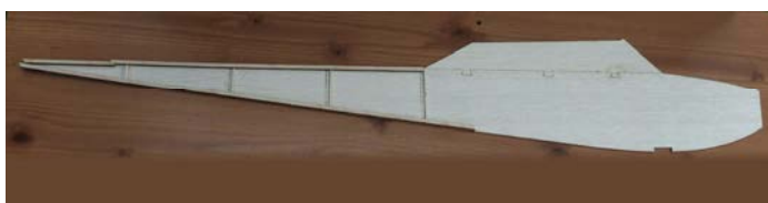
Ann added some small strips of scrap balsa to the inside of the rear fuselage to assist with the alignment of the rear formers.
