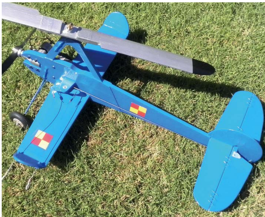
The lead outs run through the up swept tip reinforced with 1.5mm ply. Allan also added small tube guides.
