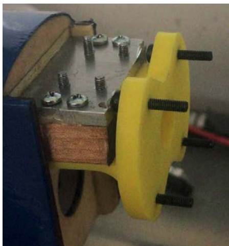
For the Nobler a motor mount was designed to allow use of the stub bearers to mount the electric motor.
