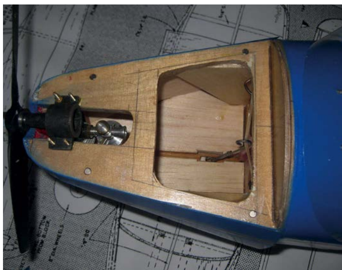
The engine compartment is cavernous but needs to be kept light; keep fretting that plywood!
