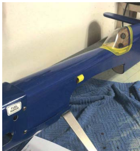
Air scoops to provide cooling for the ESC in the Nobler fuselage.
