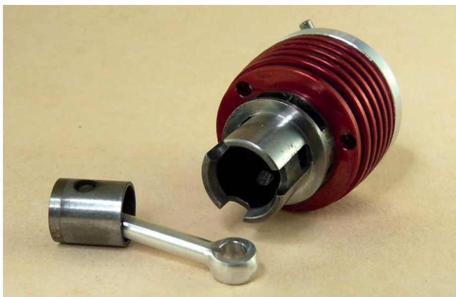
The true heart of the engine. Fins are permanently shrunk onto cylinder for excellent cooling. Porting design differs from original ED type – probably an improvement. Adequate metal all round might be part of this engine's stable performance.
