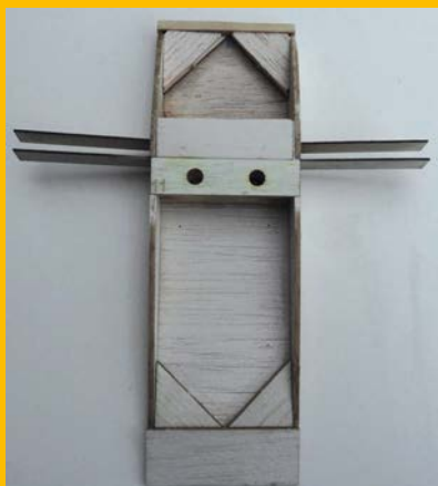
The wing centre section is constructed as a unit before the wing panels are added.
