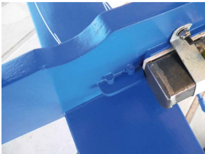
The bellcrank mount with safety dowels can be seen just behind the tank
