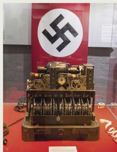
A German Lorenz cipher machine, known as Tunny by the British codebreakers
