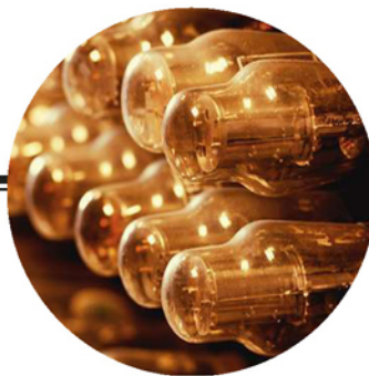
Valves on the groundbreaking Colossus codebreaking machine (see page 28)
