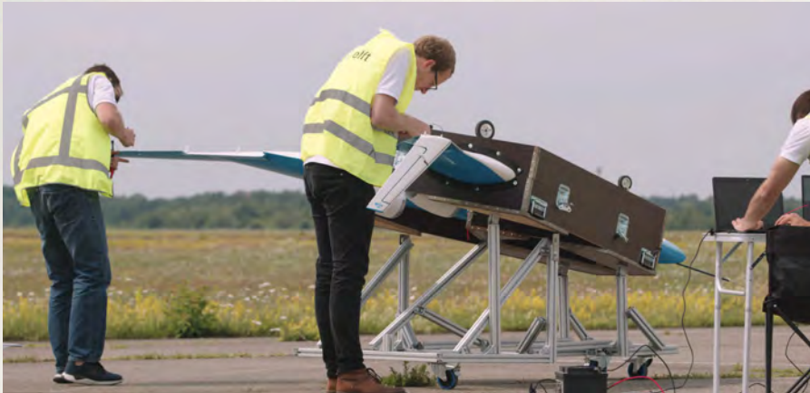
LEFT: The Dutch team has created a 22kg and 3m-wide scale model of the Flying-V Joep van Oppen
