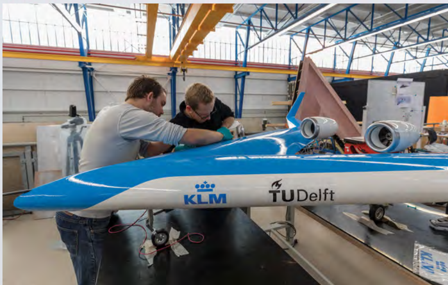
ABOVE: Engineers considered inter-engine clearance, the centre-of-gravity and aerodynamic interaction with the wing when deciding where to place the powerplants Henri Werij
