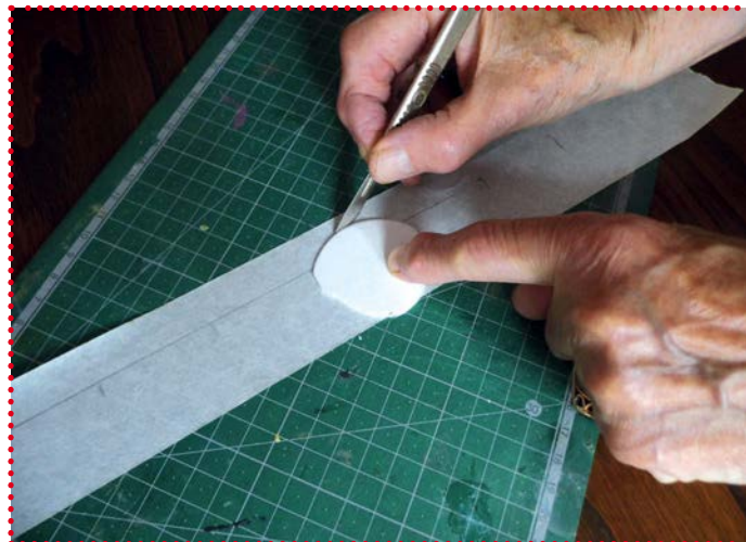
Repeatedly cut around the plastic template aligned with where the line crosses the spacing marks to produce the scallop mask.
