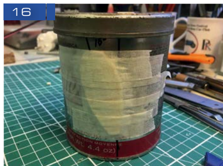
13: Adding the wing centre section reinforcements, note glue on the edges only. 14: Nose block is located with some 1/8" square balsa. 15: Propeller blades soaking in water, note 15 degree line marked on the tin. 16: Propeller blades taped to can in line with the 15 degree line to dry. 17: Cocktail sticks are cyanoed to the rear concave side of the blades. A section of ballpoint pen inner tube forms the hub. 18: Completed prop - the loop on the front allows the motor to be wound without removing the nose block.
