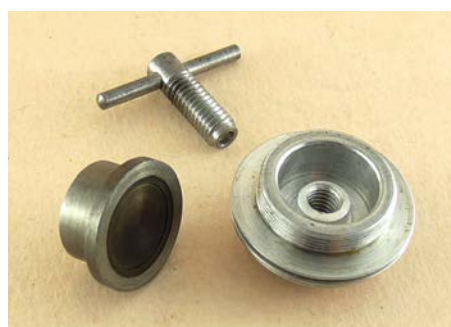
Cast iron head sleeve has cast iron contra piston. A good combination that generally gives trouble-free operation. Jon's head fits precisely onto the sleeve for good heat dissipation.
