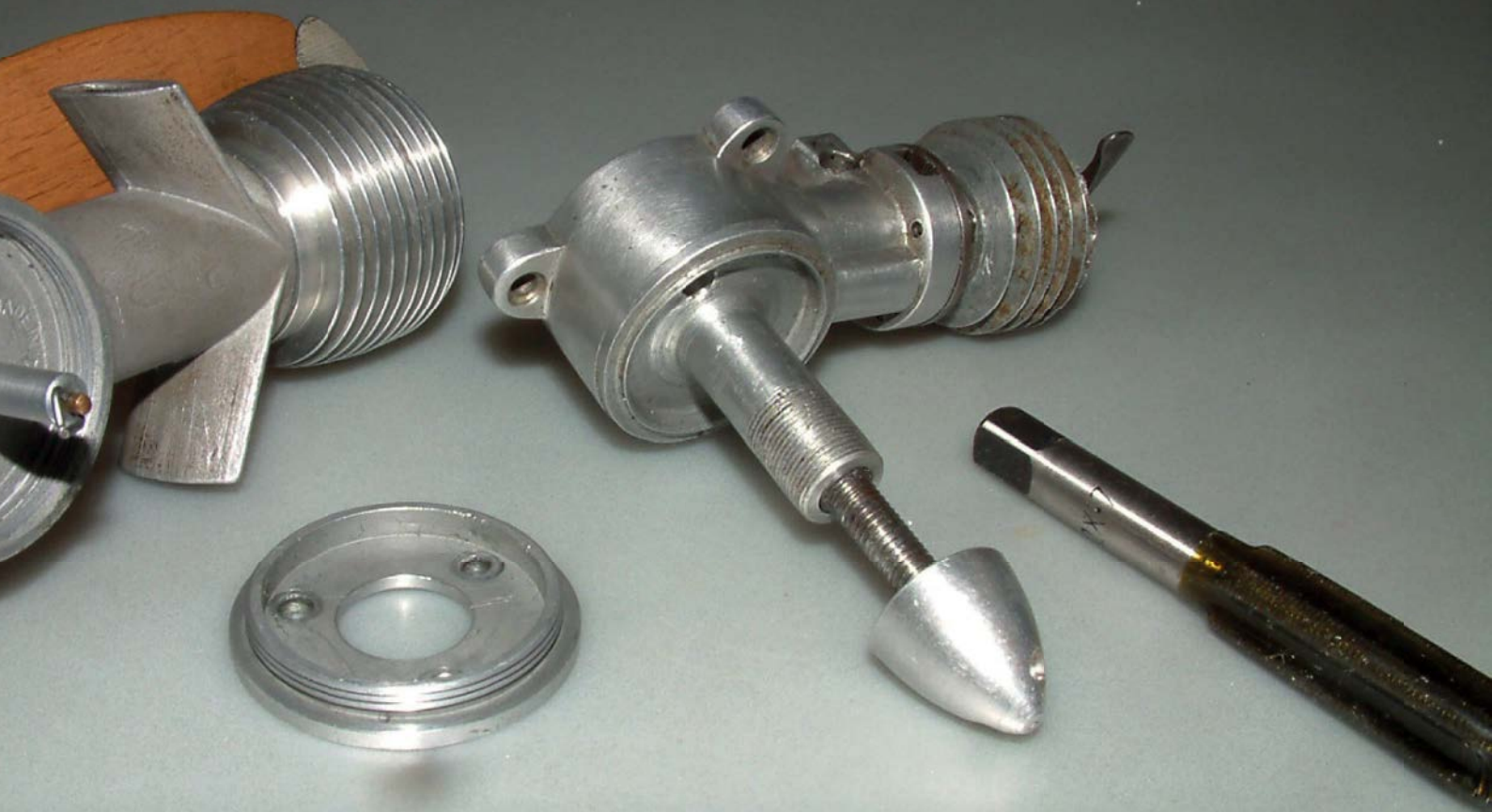
John Goodall's Antares diesel (2cc not 4cc) during restoration, the distorted top cooling fin just visible. The tap on the right has a fine 12 x 0.75mm pitch thread and was used for making the front fuel tank cup.
