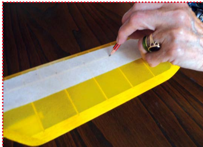
Using the model's wing to directly mark the rib spacing on to the wide tape.
