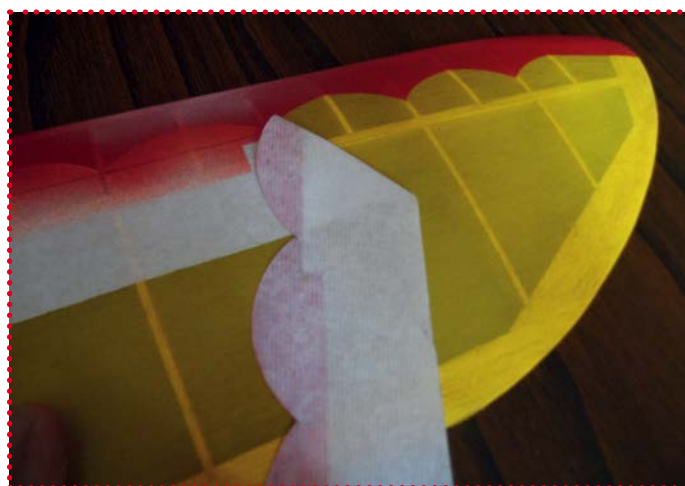
Once you have sufficient coverage of the scallop colour remove the tape, remembering to avoid smearing the paint from the tape on to the wing if it is still wet. If you are not as precise as Dave with your spraying, then newspaper at the lower edge prevents overspray.
