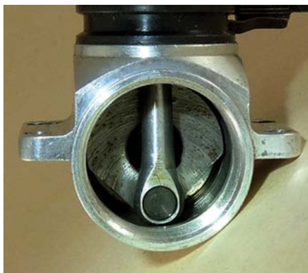
ABOVE LEFT: A peek inside shows Jon's tougher crankshaft with different counterbalance and aluminium conrod. ABOVE CENTER: Sometimes, a traditional spraybar carburettor can work better in diesels than the Cox peripheral jet design. We tried one in Jon's engine. ABOVE RIGHT: Tiny wire circlips retain the traditional wrist pin in cast iron piston. By careful machining, reciprocating mass is less than the original Cox piston/conrod assembly. An important detail for low vibration at peak speeds. The exhaust port orientation is no accident either. In theory giving a little more power, as flow into the transfer passages is easier.
