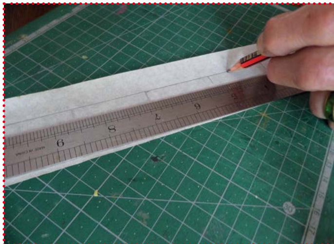
A straight line has been drawn far enough back from the top edge of the tape to allow the template to fit. To avoid over spray getting on the model the text suggests having a sheet of newspaper attached under the lower edge of the tape.
