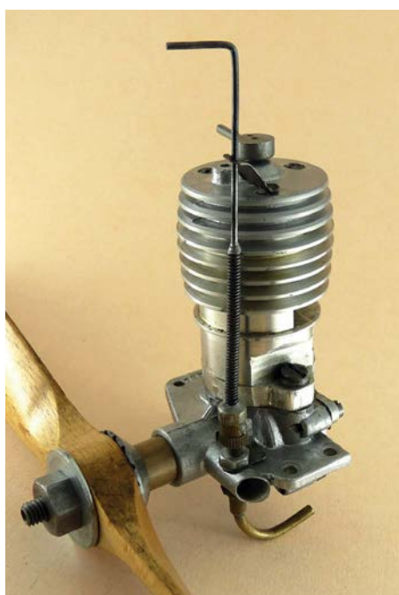
It took our stronger bar-stock cylinder barrel to revive this 1940s Comète Junior diesel, which had "blown its top" back in the day. Its spark ignition design elements couldn't stand up to diesel stress. Same goes for many glowplug engines.
