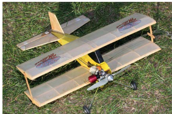
Alex Phin devised this RC RTP device to allow him to fly IC power CL (13" span Chubby biplane) in his garden on 8 foot lines(!) from outside the circle. The control uses an old 27 MHz radio he had lying around; seems sort of wrong to be checking frequency clashes when flying CL!
