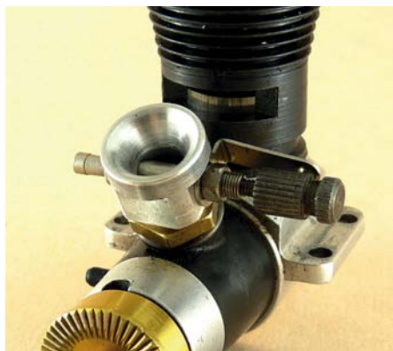
ABOVE LEFT: A peek inside shows Jon's tougher crankshaft with different counterbalance and aluminium conrod. ABOVE CENTER: Sometimes, a traditional spraybar carburettor can work better in diesels than the Cox peripheral jet design. We tried one in Jon's engine. ABOVE RIGHT: Tiny wire circlips retain the traditional wrist pin in cast iron piston. By careful machining, reciprocating mass is less than the original Cox piston/conrod assembly. An important detail for low vibration at peak speeds. The exhaust port orientation is no accident either. In theory giving a little more power, as flow into the transfer passages is easier.
