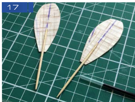
13: Adding the wing centre section reinforcements, note glue on the edges only. 14: Nose block is located with some 1/8" square balsa. 15: Propeller blades soaking in water, note 15 degree line marked on the tin. 16: Propeller blades taped to can in line with the 15 degree line to dry. 17: Cocktail sticks are cyanoed to the rear concave side of the blades. A section of ballpoint pen inner tube forms the hub. 18: Completed prop - the loop on the front allows the motor to be wound without removing the nose block.
