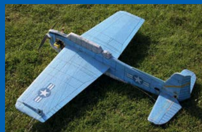
Chris Howell's semi-scale Grumman Avenger carrier deck model. It is converted from a Hobby King RC YAK 55 by reshaping around the edges and adding bits. It has already won competitions as it excels at the slow laps, although not so fast at the top end.
