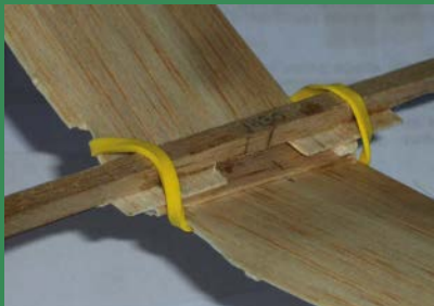
Initially the wing is held in place by a single band loop to allow repositioning during trimming. An easier peg retention system can be fitted later.
