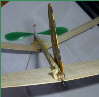
Give yourself room near the fin to attach the rubber motor to the hook.
