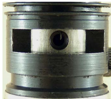
ABOVE LEFT: A peek inside shows Jon's tougher crankshaft with different counterbalance and aluminium conrod. ABOVE CENTER: Sometimes, a traditional spraybar carburettor can work better in diesels than the Cox peripheral jet design. We tried one in Jon's engine. ABOVE RIGHT: Tiny wire circlips retain the traditional wrist pin in cast iron piston. By careful machining, reciprocating mass is less than the original Cox piston/conrod assembly. An important detail for low vibration at peak speeds. The exhaust port orientation is no accident either. In theory giving a little more power, as flow into the transfer passages is easier.
