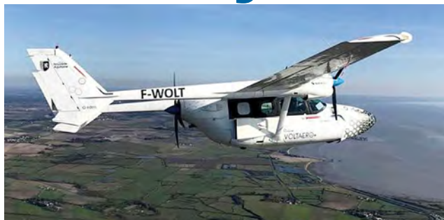
The Cessna 337-based Cassio 1 testbed during its maiden flight on October 11 after installation of the new hybrid-electric powertrain designed for the ten-seat Cassio 600 VoltAero
