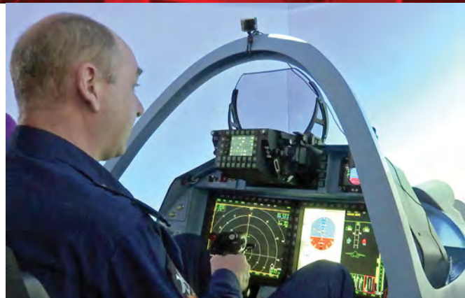
The Su-57's cockpit features two large MFI-50 displays, small MFPI-50 display and control panel, and a ShkAI-50 head-up display Russian MoD
