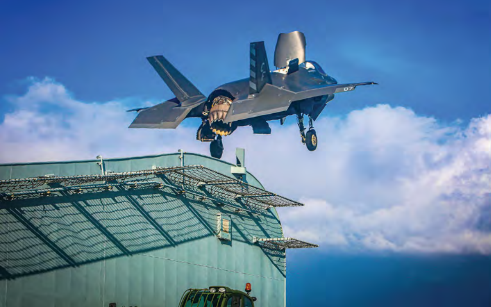
CLOCKWISE FROM LEFT: F-35B 169608/CF-07 departs the Queen Elizabeth with the nozzle of its Pratt & Whitney F135 engine pointing downwards, providing the push to get it off the deck 3 MAW/1st Lt Zachary Bodner
