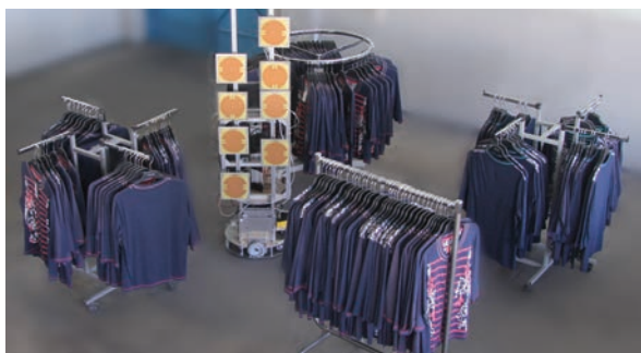
Figure 16. A mobile robot platform equipped with a UHF-RFID MIMO system drives autonomously through a real warehouse scenario and streams the tag data to a computer, where the localization algorithm estimates the real tag positions.
