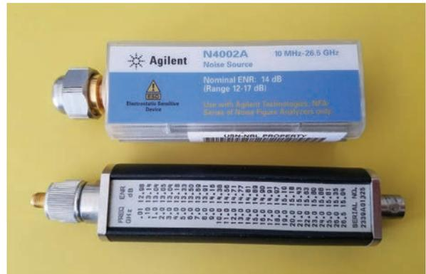
**Figure 6.** Standard noise sources in the microwave range. The most recent offering (top) will carry the ENR information electronically and provide it to the instrument automatically via USB cable.
