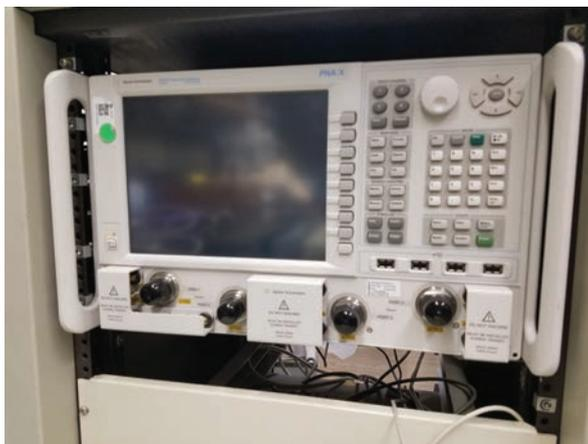
**Figure 5.** A modern noise figure meter integrated as a personality of a vector network analyzer.
