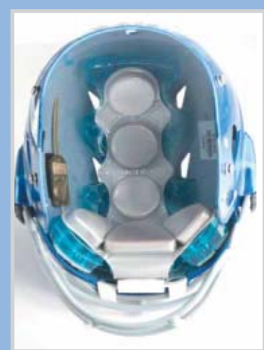
Hothead Technologies has developed sensor equipment that can be installed in a football helmet to warn that a player may be about to suffer heatstroke.
