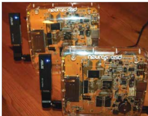
Figure 4. Prototype implementation using Neuros OSD boards.
