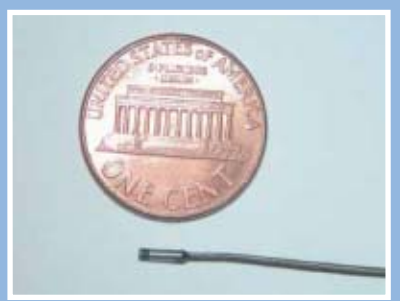
Two Israeli companies have developed the world's smallest medical camera, the IntroSpicio 120, shown here next to a US penny.
