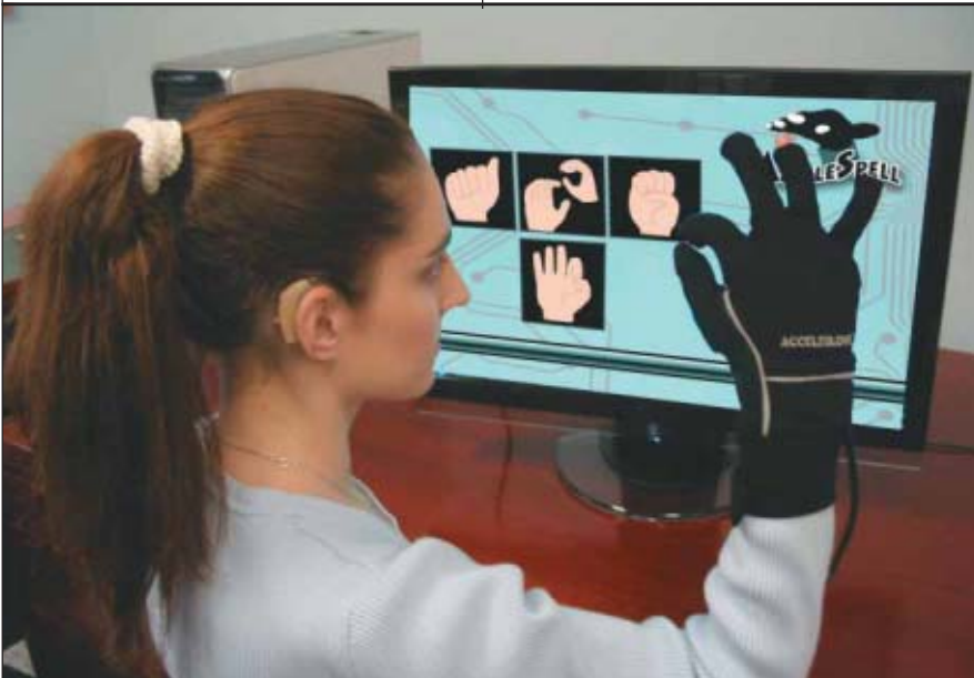
AnthroTronix has released a programmable data glove that records users' hand and finger motions to let them interact in novel ways with computer systems. In this case, the user is using the AcceleGlove to play a game that requires communication via sign language.
